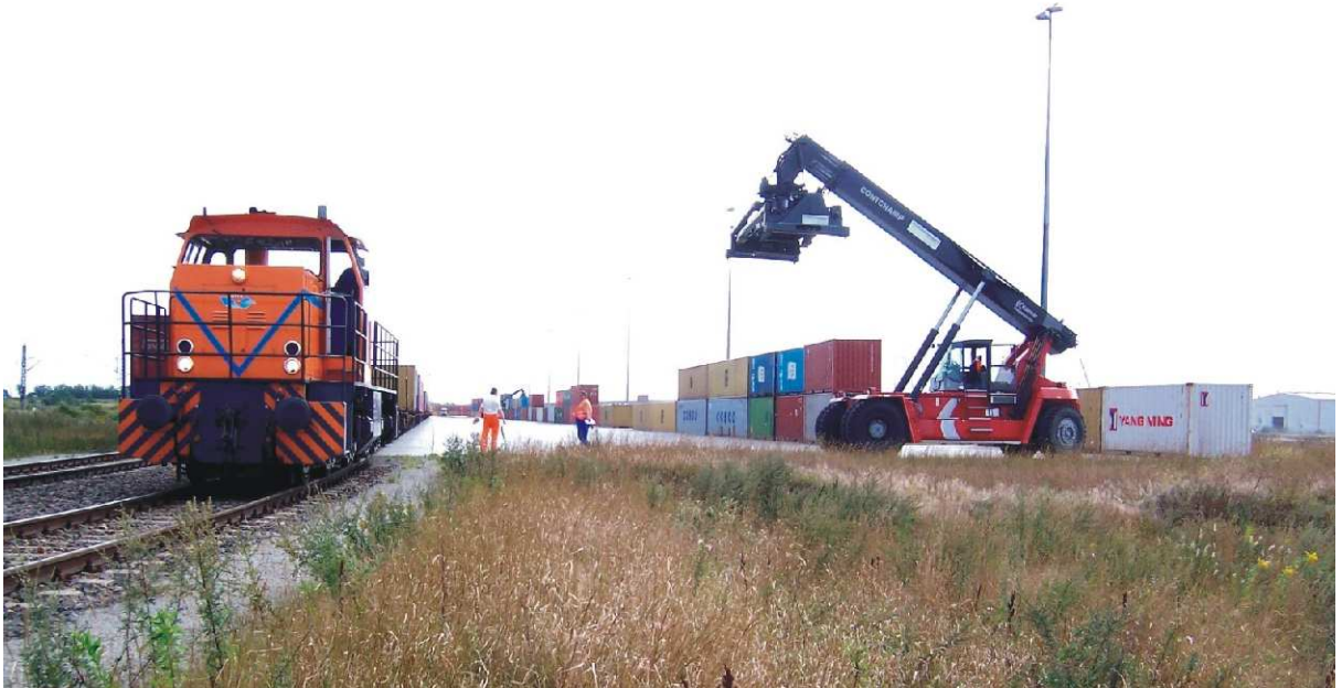
Cargo handling terminal in the GVZ Berlin West change from road to railway
